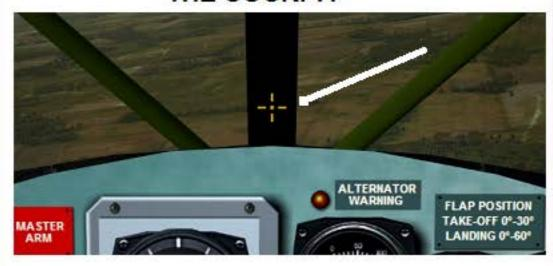
A Nose-cross can be superimposed on the cockpit graphic, by use of the HUD controls, to aid in orientation.
