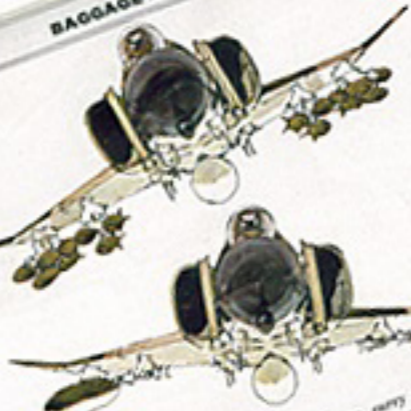
F-4 holds 3,300 gallons of fuel, most modern with aerial tanker to top tanks going in and out of North Vietnam. Spad hold thirty gallons.
